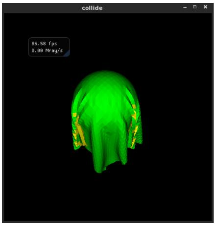
This tutorial demonstrates how to implement collision detection using the collide API. A simple cloth solver is setup to collide with a sphere.
