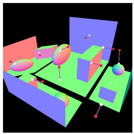
This tutorial demonstrates a use-case of the point query API. The scene consists of a simple collection of objects that are instanced and for several point in the scene (red points) the closest point on the surfaces of the scene are computed (white points). The closest point functionality is implemented for Embree internal and for user-defined instancing. The tutorial also illustrates how to handle instance transformations that are not similarity transforms.
