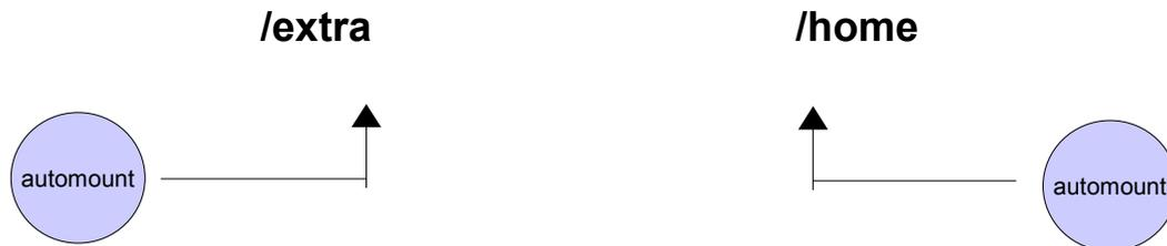
When **autofs** is started it will invoke an instance of **/usr/sbin/automount** for each mount point defined in the master map **/etc/auto.master**.
