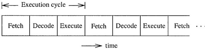
Figure 4.1 Execution cycle of a typical computer system.
