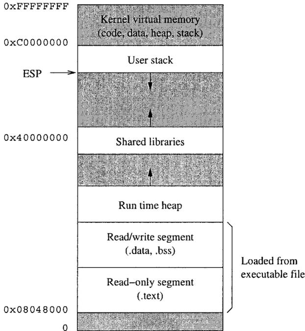
Figure 12.6 Memory layout of a Linux process.
