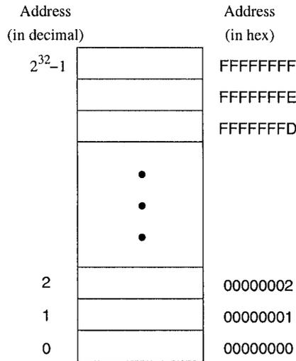
**Figure 3.1** Logical view of the system memory.
