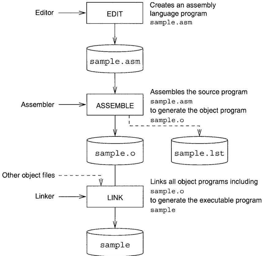
**Figure 7.2** Assembling and linking assembly language programs (optional inputs and outputs are shown by dashed lines).
