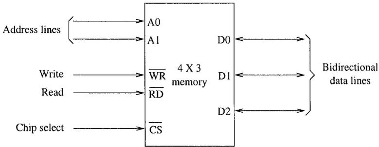
Figure 3.5 Block diagram representation of a  $4 \times 3$  memory.
