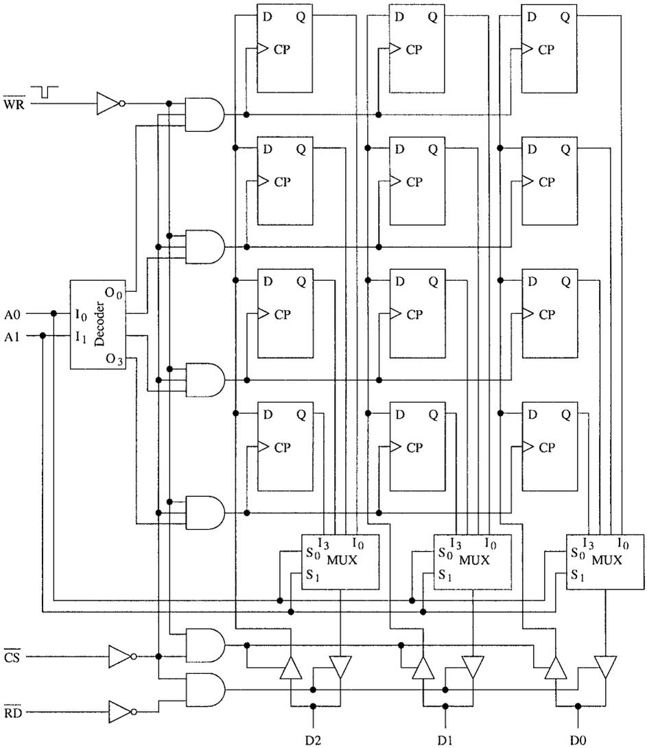
Figure 3.4 A 4 × 3 memory design using D flip-flops.
