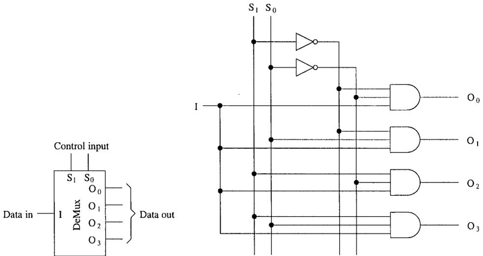
**Figure 2.13** Demultiplexer block diagram and its implementation.
