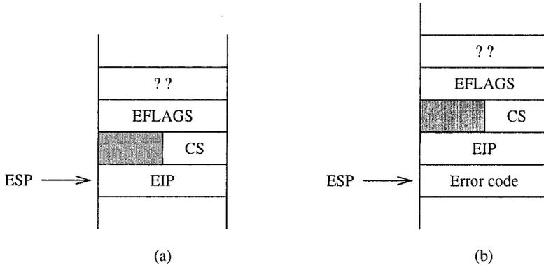
Figure 20.5 Stack state after an interrupt invocation.
