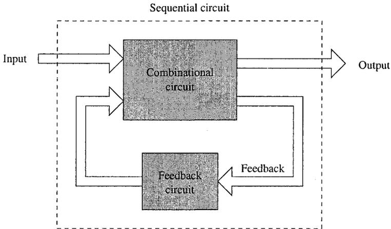
Figure 2.25 Main components of a sequential circuit.
