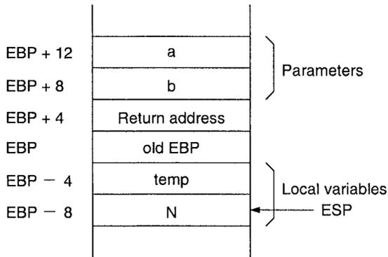
**Figure 12.1** Activation record for the `compute` function.
