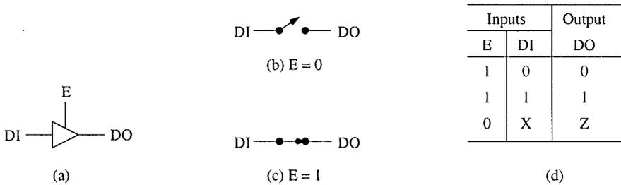
**Figure 3.3** Tristate buffer: (a) logic symbol; (b) it acts as an open circuit when the enable input is inactive ( $E = 0$ ); (c) it acts as a closed circuit when the enable input is active ( $E = 1$ ); (d) truth table ( $X$  = don't care input, and  $Z$  = high impedance state).
