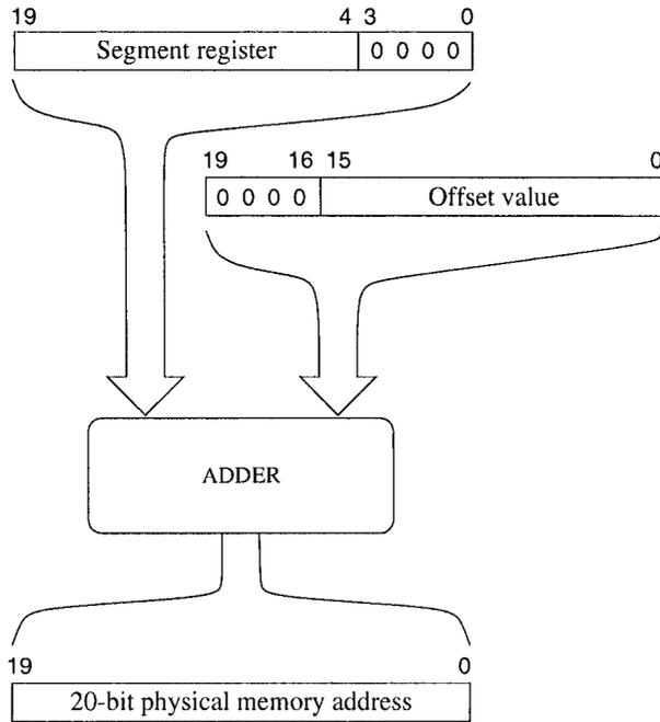
**Figure 4.12** Physical address generation in the real mode.
