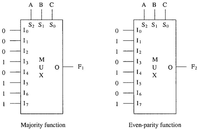
Figure 2.12 Two example implementations using an 8-to-1 multiplexer.
