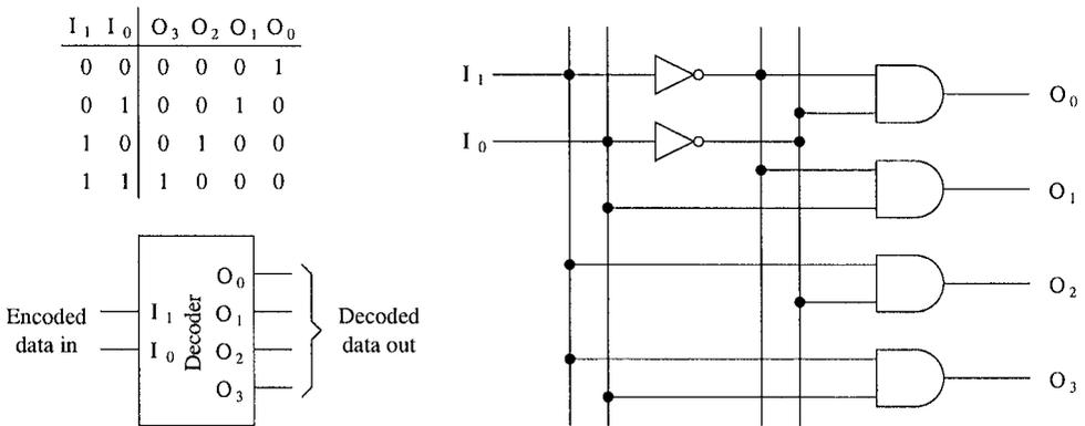
Figure 2.14 Decoder block diagram and its implementation.
