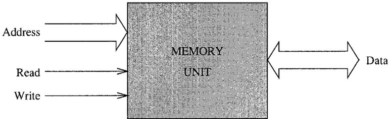
**Figure 3.2** Block diagram of the system memory.
