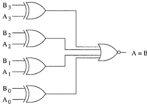
Figure 2.15 A 4-bit comparator implementation using XOR gates.
