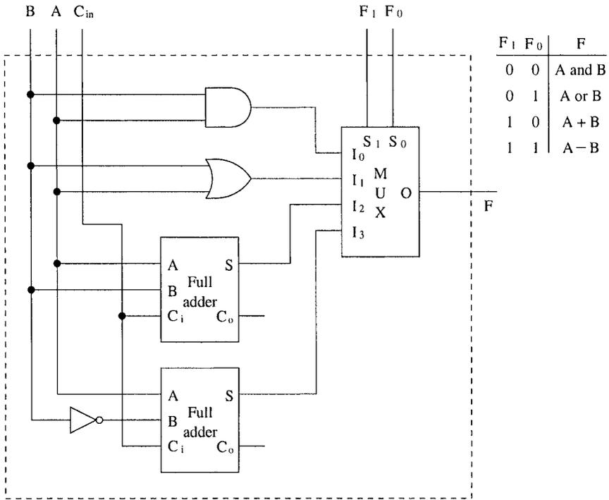
**Figure 2.22** A simple 1-bit ALU that can perform addition, subtraction, AND, and OR operations. The carry output of the circuit is incomplete in this figure as a better and more efficient circuit is shown in the next figure. Note: “+” and “-” represent arithmetic addition and subtraction operations, respectively.
