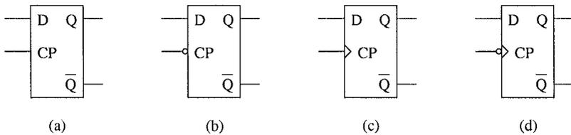
**Figure 2.30** Logic symbol notation for latches and flip-flops: (a) high level-sensitive latch; (b) low level-sensitive latch; (c) positive edge-triggered flip-flop; (d) negative edge-triggered flip-flop.
