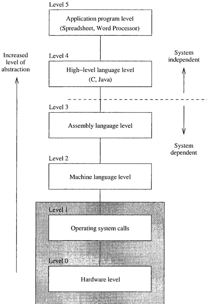
**Figure 1.1** A user's view of a computer system.
