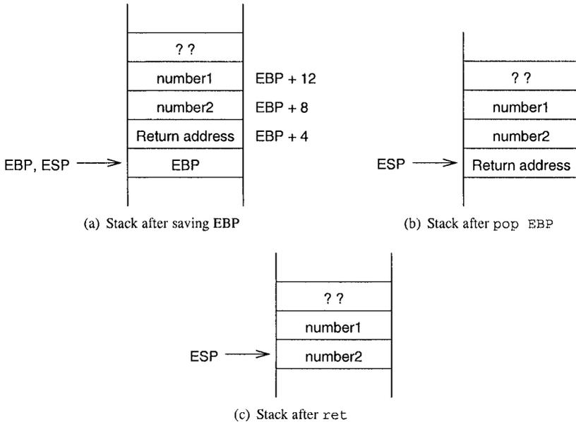
**Figure 11.8** Changes in stack state during a procedure execution.
