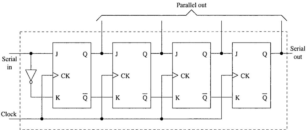
**Figure 2.32** A 4-bit shift register using JK flip-flops.
