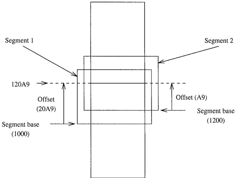
**Figure 4.13** Two logical addresses map to the same physical address (all numbers are in hex).
