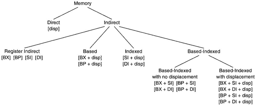
Figure 13.1 Memory addressing modes for 16-bit addresses.
