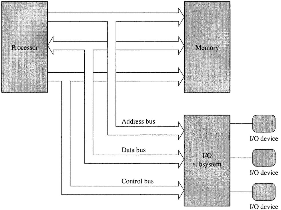
**Figure 2.1** Simplified block diagram of a computer system.
